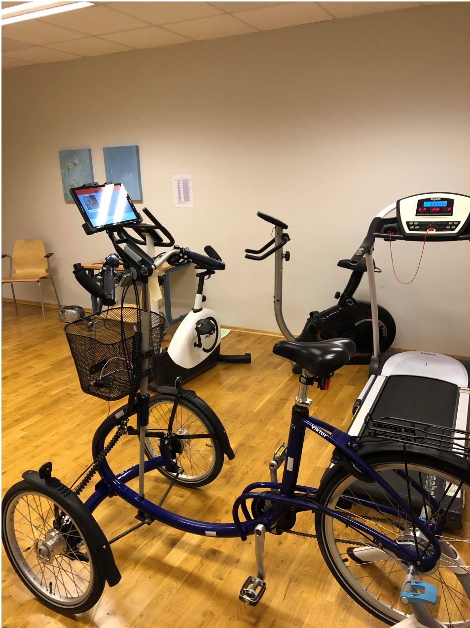
Figure 2.5: Tacx Smart Flow trainer with three-wheel bicycle and tablet
