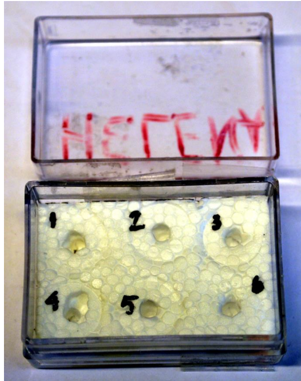
Figure 1. Container (3.5 × 5 cm) with lid, prepared with Styrofoam and holes for the scanning electron microscope (SEM) specimen stubs. This specific container can hold up to six stubs.
