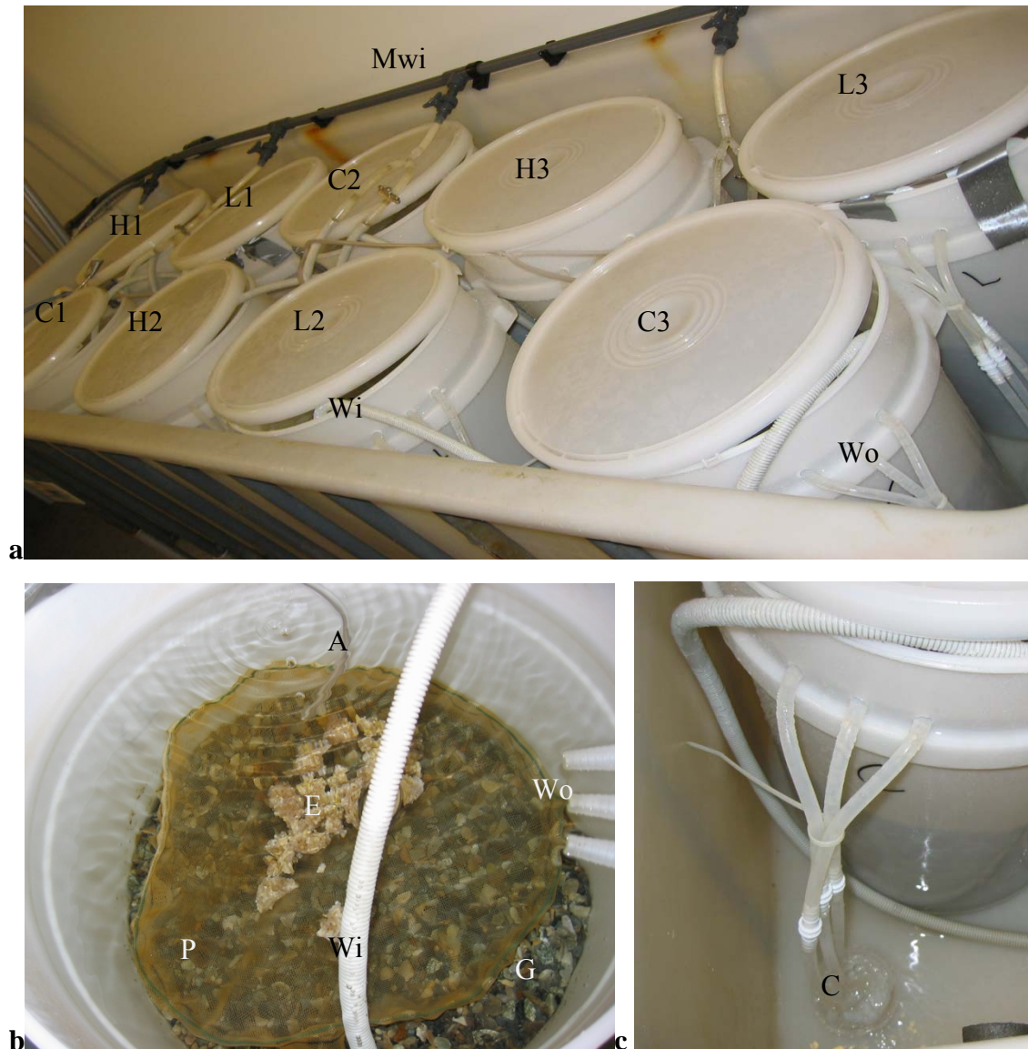
Figure 1. Experimental design. Photo a, Each experimental unit with lids on marked with treatment code (C= Control, L= low dose, H= High dose oil), main water inlet (Mwi) and container water inlet (Wi) and water outlet with three tubes (Wo). Photo b, the experimental units viewed from above: Plankton netting dish (P), Water inlet (Wi), Water outlet (Wo), Eggs (E) on the plankton net, Air supply (A) and Gravel (G). Photo c, Smaller Cups with plankton nets (C) to collect larvae escaping the main container.
