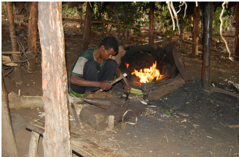
Fig 10. Blacksmith sitting on Chefat made of leaves and use chembina to protect the handle of the knife from the hot fire
