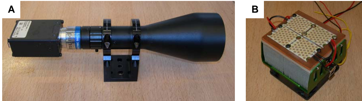
Figure 9. Camera with telecentric lens (A) and LED-array used for backlighting (B), mounted on a computer fan for cooling.
