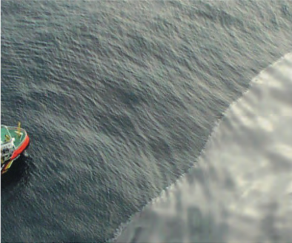
Figure 4.8: Image showing the change in surface roughness between areas of open ocean and slick infested areas. As can be seen, small-scale undulations are less prevalent within the slick but large-scale surface undulations are preserved across both scattering surfaces. Taken from [ITOPF, 2011 (a)].
