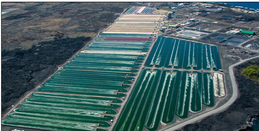
Figure 5: Cultivation of microalgae in race-way ponds. Photo credit: Cyanotech corporation. Reproduced with permission.
