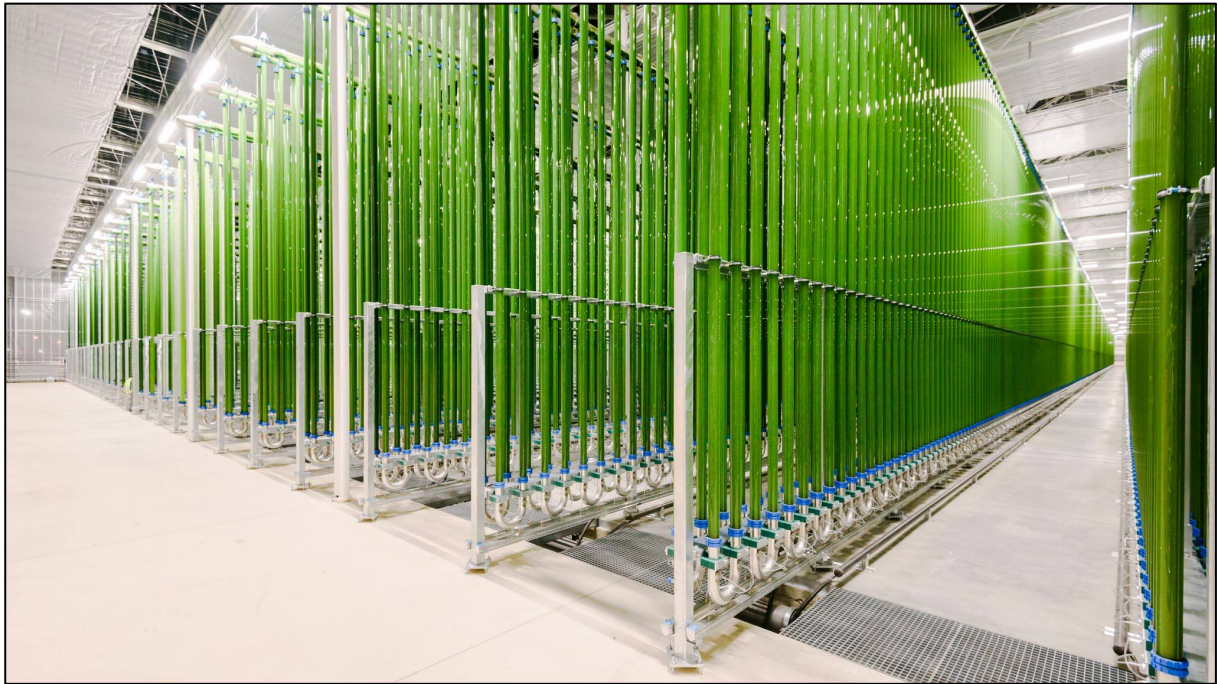
Figure 6: Cultivation of microalgae in glass tubes. Photo credit: Ecoduna AG. Reproduced with permission.
