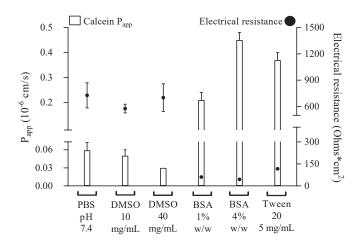
**Fig. 2.** PVPA barrier integrity expressed as apparent permeability ( $P_{app}$ ) of calcein (5.5 mM) and electrical resistance across the barriers with different media in the acceptor compartment, and calcein 5.5 mM in the donor compartment (in PBS pH 6.5). (Mean  $\pm$  SD; n = 12).
