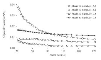
Fig. 1. Viscosity of mucus at different pH conditions (5.5, 6.2 and 7.4) and mucin concentrations (10 mg/mL and 40 mg/mL).
