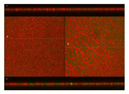
**Fig. S3.** Confocal laser scanning microscopy of the PVPA barrier labelled with rhodamine (red) after soaking for 3 hours in mucin 40 mg/mL marked with calcein (green). The two micrographs were taken from two different positions in the barrier. The white lines mark the placement of the cross-sections a and b shown at the top and bottom, respectively.
