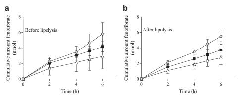
**Fig. 5.** Cumulative amount of fenofibrate permeated across the mucus-PVPA barriers from super-SNEDDS solution<sub>150</sub> (grey circle), SNEDDS<sub>75</sub> (black square) and super-SNEDDS suspension<sub>150</sub> (white triangle) A) before (0 min) and B) after (30 min) lipolysis. (Mean  $\pm$  SD; n = 6).
