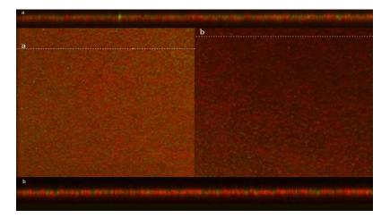
**Fig. S1.** Confocal laser scanning microscopy of the PVPA barrier labelled with rhodamine (red) after soaking for 3 hours in calcein solution (green). The two micrographs were taken from two different positions in the barrier. The white lines mark the placement of the cross-sections a and b shown at the top and bottom, respectively.
