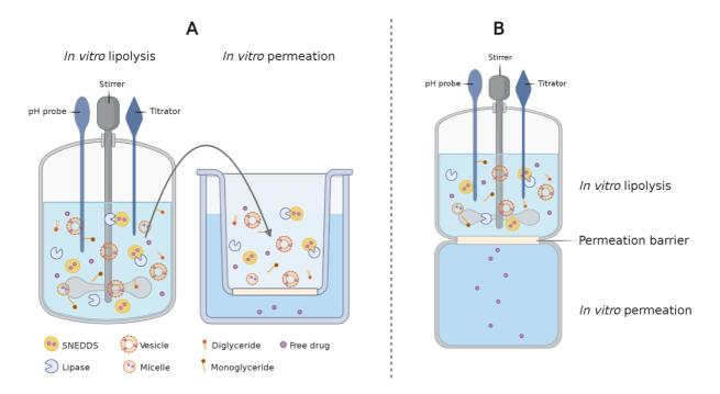
Figure 1.17: A) Combined and B) simultaneous in vitro lipolysis-permeation models.
