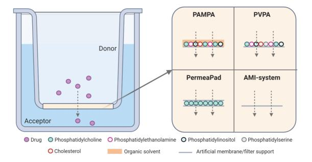
**Figure 1.14**: *In vitro* permeability setup, composed of a donor and acceptor compartment, separated by a permeation membrane. The main cell-free permeation membranes: PAMPA, PVPA, PermeaPad<sup>®</sup> and AMI-system.
