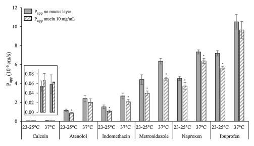
**Fig. 5.** Permeability of different compounds in the presence and absence of mucin (10 mg/mL) at room temperature (23–25 °C) and at 37 °C. The results are indicated as mean  $\pm$  SD (n=3). Statistical significance (p < 0.05) was investigated with one-way ANOVA using the Bonferroni *post hoc* test. \*Statistically significant difference in drugs' P<sub>app</sub> in
