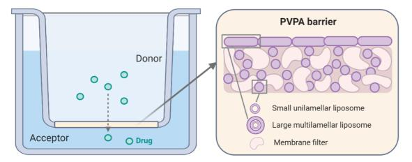
**Figure 1.15**: Structure of the PVPA barriers, composed of small unilamellar and large multilamellar liposomes immobilized in and on top of a membrane filter.
