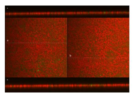
**Fig. S2**. Confocal laser scanning microscopy of the PVPA barrier labelled with rhodamine (red) after soaking for 3 hours in mucin 10 mg/mL marked with calcein (green). The two micrographs were taken from two different positions in the barrier. The white lines mark the placement of the cross-sections a and b shown at the top and bottom, respectively.
