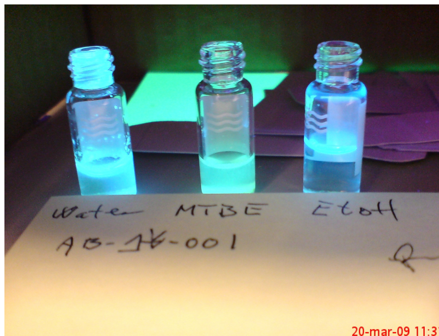
Figure 3.4 2,4,6- triphenylpyrylium tetrafluoroborate dissolved in different solvents under long wave UV radiation. Studies on this fluorescent effect of pyrylium salts show that it is highly dependent upon how the counterion interacts with the pyrylium.
