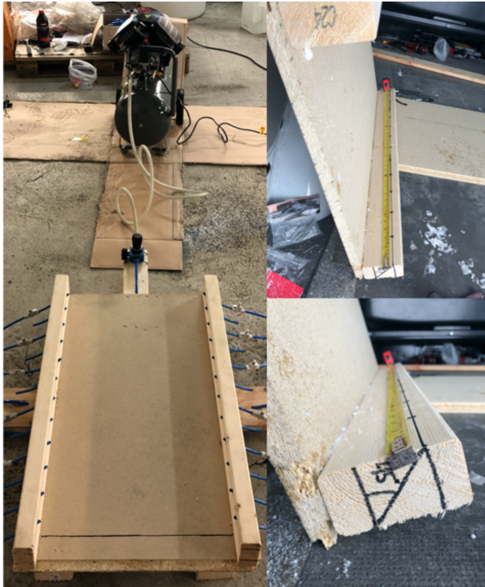
Figure 38: Boards with drilled holes for outlets
