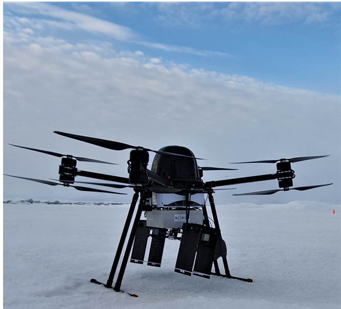
(c) Antenna prototype (and radar box) mounted under "Cryocopter FOX." The antenna angle regulation mechanism has a slight angle when not powered up to ensure tension on stabilizing bungees when pointing in nadir.
