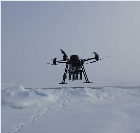
Fig. 2. UWiBaSS mounted under the UAV Cryocopter FOX during flight.
