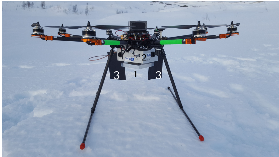
(b) Radar system mounted on an octocopter drone (Kraken), with the transmitting spiral antenna (1) mounted below the radar box (2), and the two receiving Vivaldi antennas (3) in 90 degrees offset on the sides.
