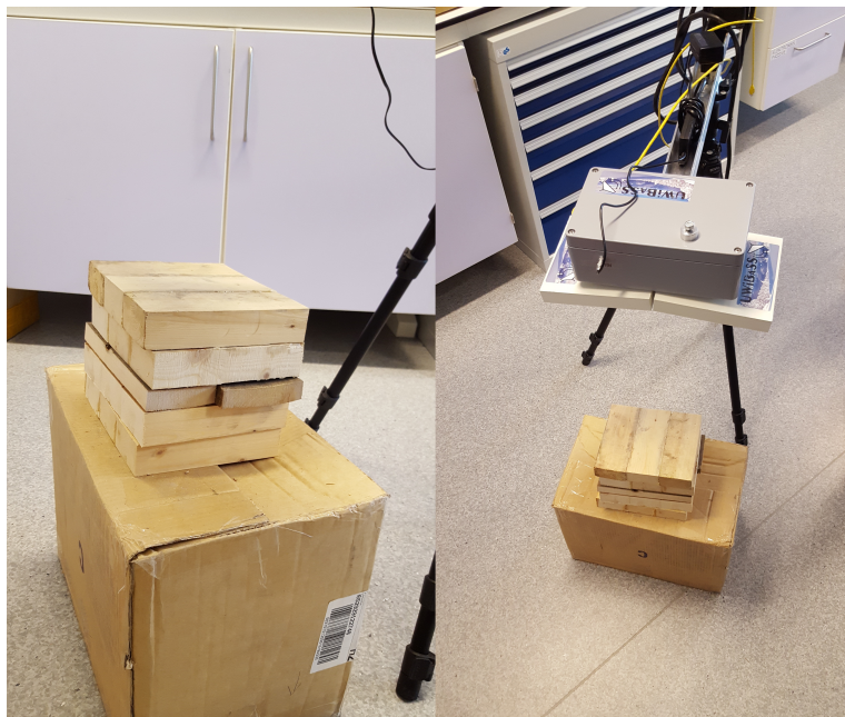
Figure A.5: Wood block, where the two darker pieces of wood were switched between wet and dry wood.
