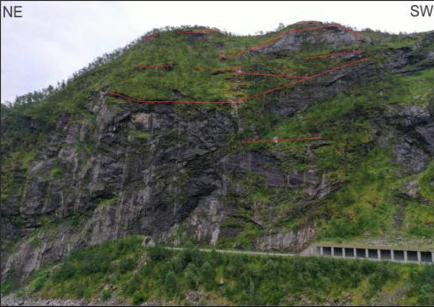
Figure 35. Drone image with the release areas (red lines) used in the modelling are shown.
