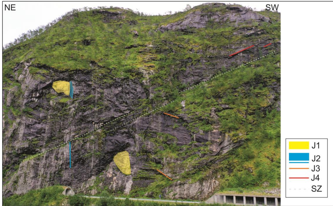
Figure 29. Drone image with illustrations of the main joints sets (J1-4) and the SZ that strikes through the cliff.
