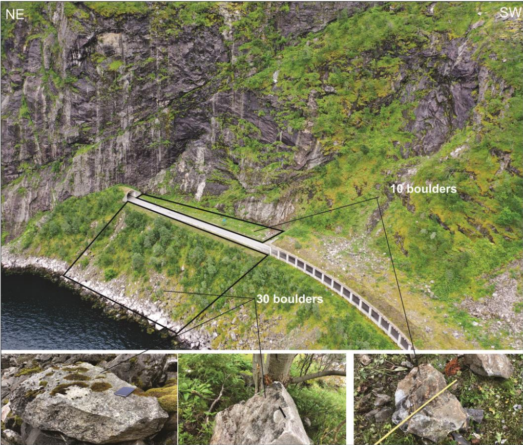
Figure 26. Drone image of the area (black polygon) where the boulders were mapped, 30 were mapped below- and ten above the road. Below drone image are examples of boulders that were mapped. These boulders were used in the numerical modelling.
