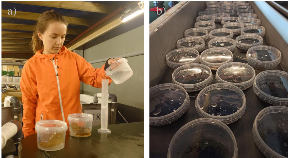
Figure 9: a) Measurement and dilution of stock solutions into beakers. b) Beakers placed randomly into the open tank with running water for temperature regulation.
