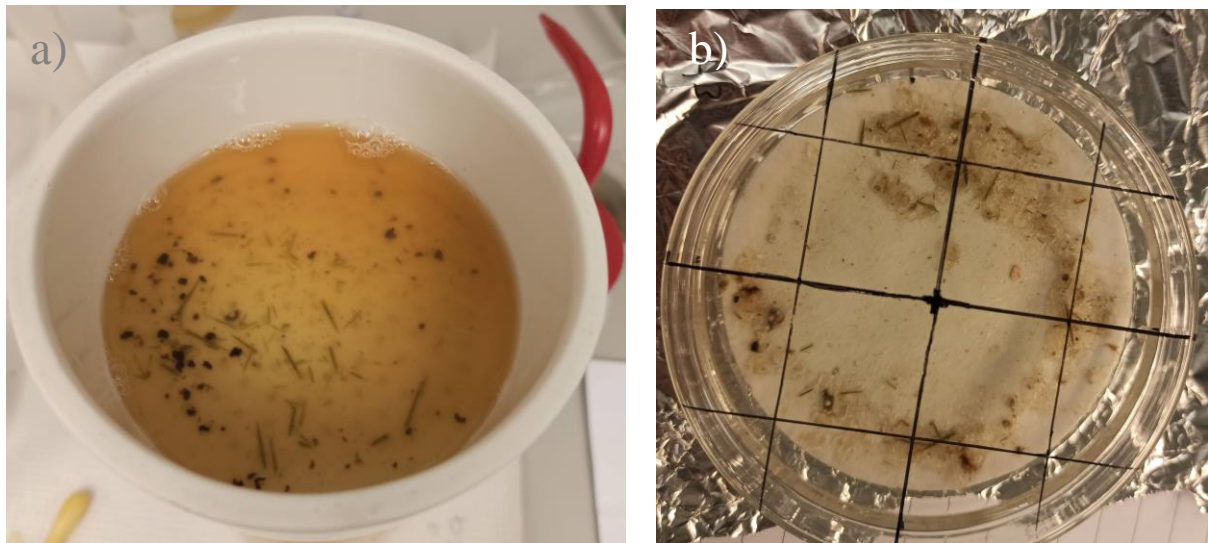
Figure 16: a) Filtration of digested intestine contents over glass microfiber filter using ceramic Büchner funnel. b) Filter analysis showing method of petri dish placed on top with drawn on division into sections
