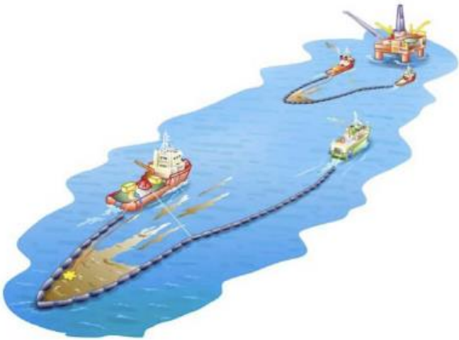
Figure 2-18 Oil containment using booms (DNV GL, 2015)
