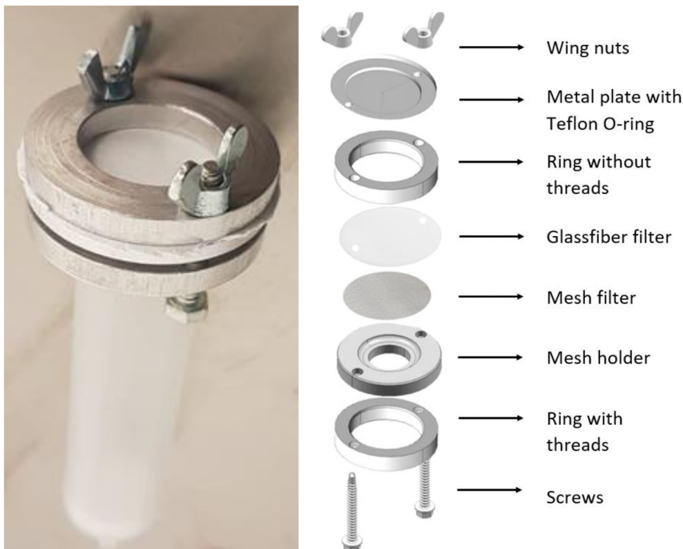
Fig. 1. Active air sampler used to collect both the gas and particle phase of the CPs. Left the modified sampler and right the schematic overview of the sampler template.
