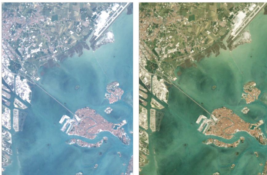
Figure 2.6: Before (left) and after (right) atmospheric correction of a Landsat-8 image of Venice, Italy, by the NASA-developed LEDAPS correction scheme. Image courtesy of Mapbox (2013).
