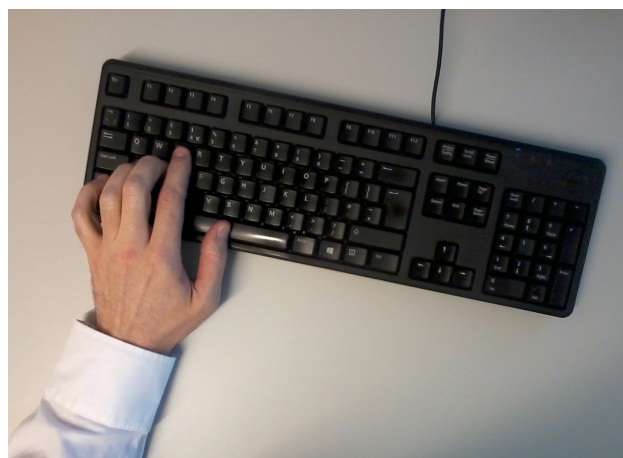
Figure 4. Hand position for the left-hand key set, with the keyboard at an angle of 10–15° to minimise finger reach strain.
