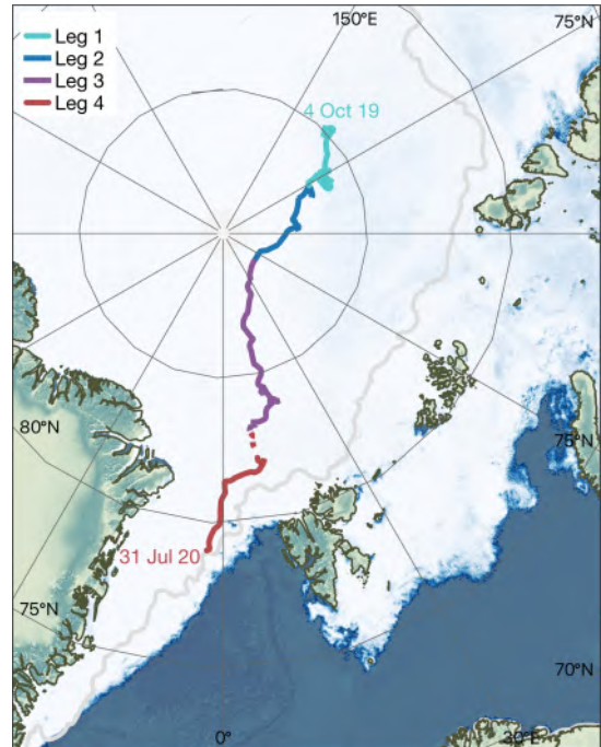
Fig. 1: Drift trajectory for the MOSAiC floe 1. The dashed line marks the time when R/V Polarstern had to leave the floe. The background shows sea ice concentration from AMSR2 (ASI 89 GHz, University of Bremen) on 3 March 2020, the maximum ice extent during the drift. The grey line marks the ice extent on 31 July 2020 at the end of floe 1.
