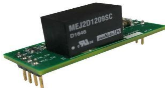
Figure 7-2: Gate Driver Cree's CGD15SG00D2 [66]
