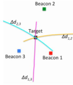
Figure 35: Visualization of TDOA method (2D space)
