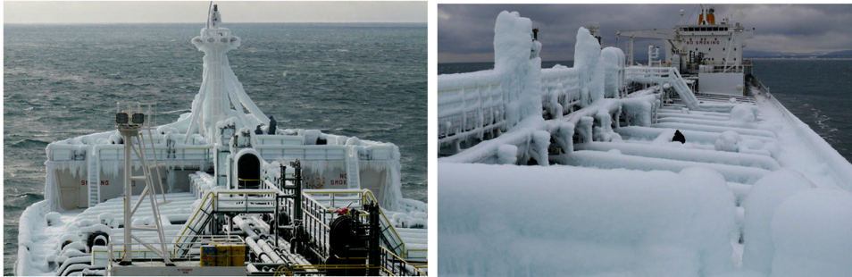
Figure 10: Sea spray icing on ships [6]
