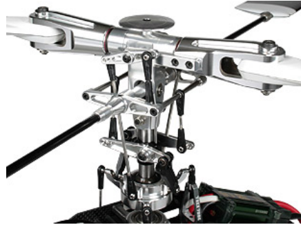
Figure 13: Helicopter swashplate setup
