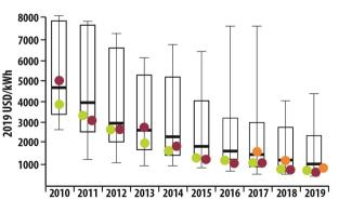
**FIGURE 4** Average LCOE (left) and CapEx (right) for Chinese, Indian and gulf utility PV projects by year. Modified box & whisker plots represent global market where boxes encompass the fifth to 95th percentile values [Colour figure can be viewed at wileyonlinelibrary.com]
