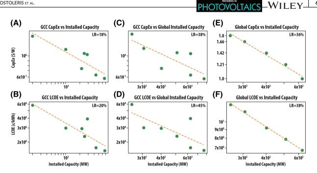
FIGURE 5 Learning curves for CapEx and LCOE for the GCC market (A.B); GCC prices versus global installations (C.D); and the global market (E,F). The learning rate is the percent reduction in cost per doubling of capacity [Colour figure can be viewed at wileyonlinelibrary.com]
