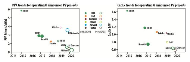
**FIGURE 1** Evolution of reported PPA prices (left) and project CapEx (right) for operating and announced/under construction utility PV projects in the GCC region [Colour figure can be viewed at wileyonlinelibrary.com]
