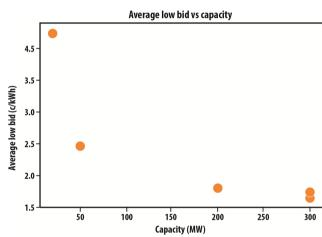
**FIGURE 3** Average of two lowest bids for five out of six PV projects tendered in Saudi Arabia's REPDO 2 auction. Evidence of economies of scale for projects below 100 MW is clear, whereas evidence for economies of scale above this level is inconclusive, although a stronger case may be made by the impending announcement of the PPA for the 600-MW Faisaliah project [Colour figure can be viewed at wileyonlinelibrary.com]
