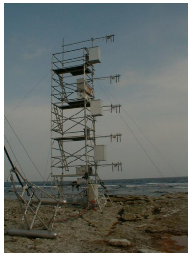
Figure 1.9: Measurements of concentrations of e.g. \text{NH}_3 in several heights can provide the basis for calculating the deposition using the Gradient method. This particular tower with measurements in 5 heights (the small grey tubes contain denuders for sampling concentrations) was operated at the island of Gotland in 1998. (Picture kindly provided by Bjarne Jensen, National Environmental Research Institute).
