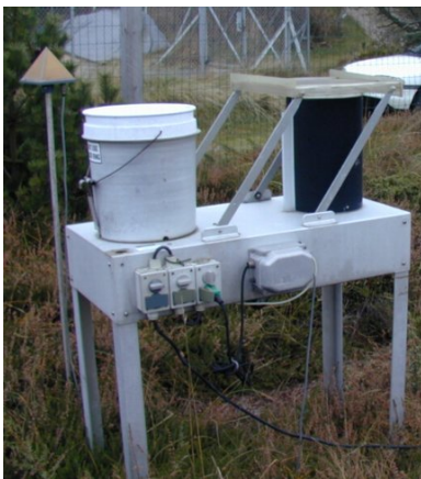
Figure 1.8: An example of a wet-only sampler applied in the Danish Background Monitoring Programme. The black bucket contains the bottle where the precipitation is sampled. A motor is located inside the top of the white table and this is used to move the lid (positioned on top of the sampling bucket in the picture). The white bucket acts as a rest for the lid when it is raining. To the left of the lid is seen the sensor that controls the position of the lid. (Picture kindly provided by Dr. Thomas Ellermann, National Environmental Research Institute).
