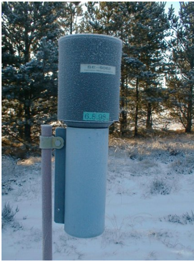
Figure 1.7: An example of a bulk sampler applied in the Danish Background Monitoring Programme. The bottle collecting the precipitation is located inside the grey tube beneath the funnel (black). (Picture kindly provided by Dr. Thomas Ellermann, National Environmental Research Institute).
