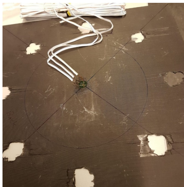
Figure 4. The rosette strain gauge attached to the back of the CFRP sample.
