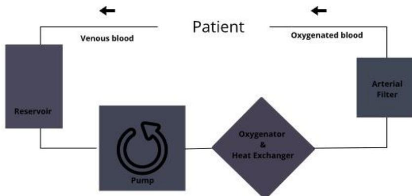
**Figure 4** - Schematic of the CPB circuit
