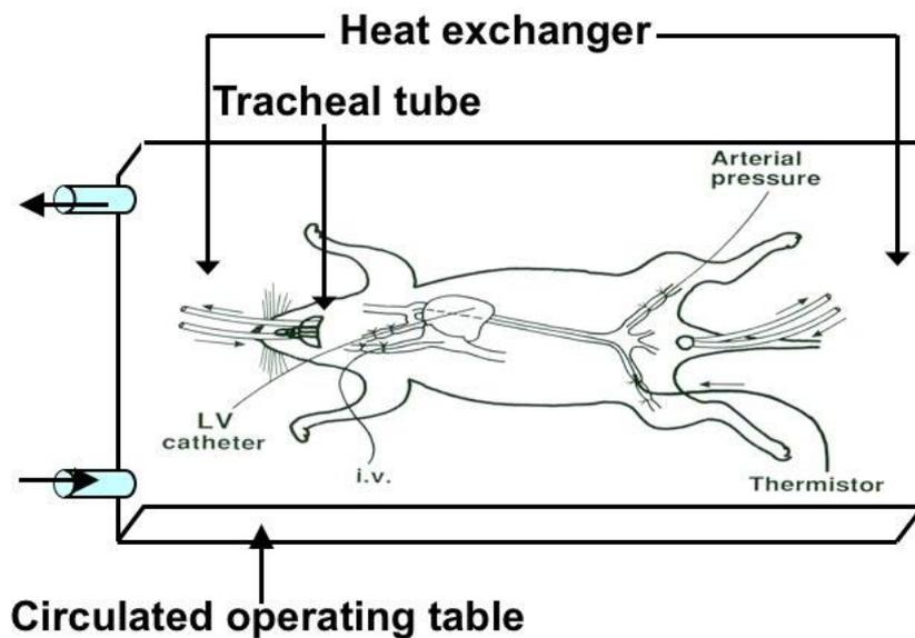
**Figure 9** - Experimental setup rat model.
