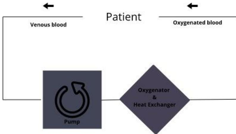
**Figure 5** - Schematic of the ECMO circuit
