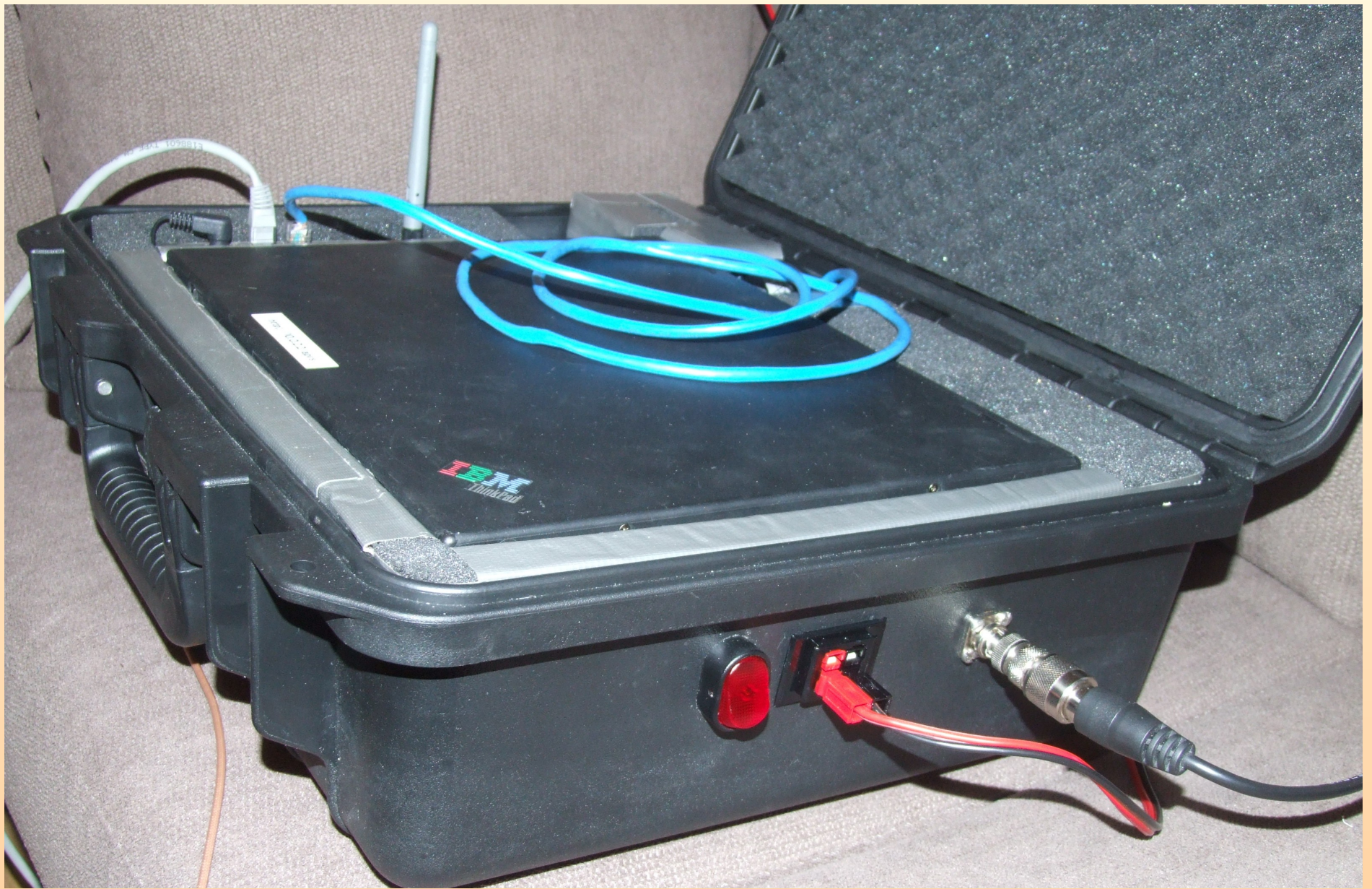
Server in a case (wireless LAN, tracker, radio, Linux PC, 12V ext. power)
