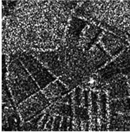
Figure 2.8: Example of the appearance of the speckle pattern in a radar image.
