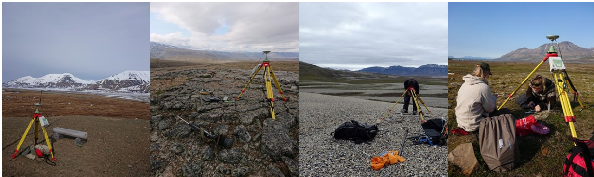
Figure 9: Leica GS10 Basestations at four locations in Svalbard used as reference point for drone flights and ground truthing. From left to right: “flagpost location”, Janssonhaugen, Sassendalen, Todalen. Pictures taken by I.Eischeid (1,2,4) and T.Blæsterdalen (3).
