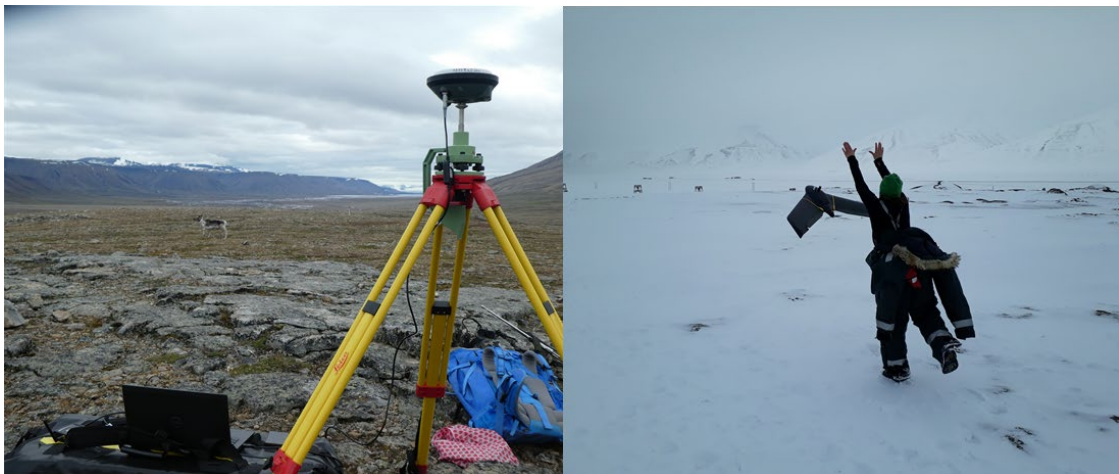
Figure 11: left: Leica GS16 basestation connected to PC (with installed eMotion (sensefly) flying software) via Leica GEV 269 cable, picture taken by I.Eischeid. Fixed wing drone (eBeeX) launch by an eager PhD student, picture by V.Ravolainen, Svalbard 2019.
