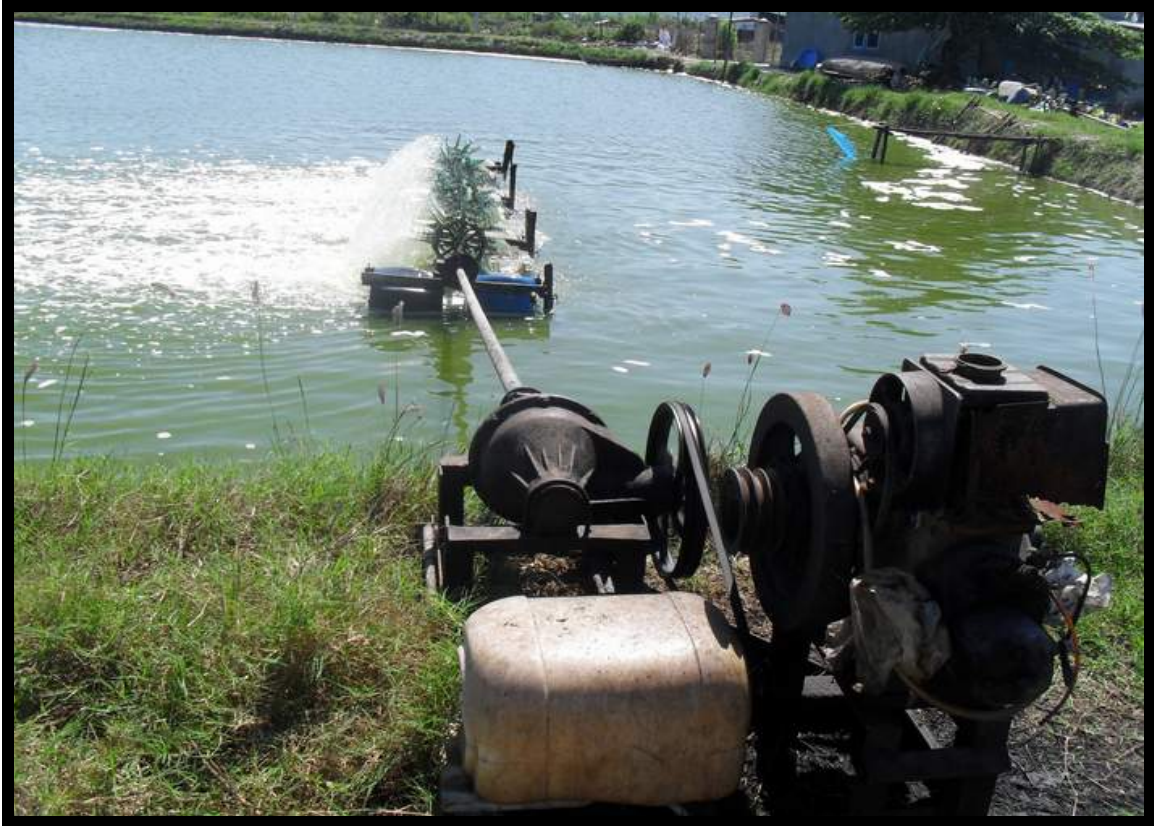
Figure 4 Using Equipment (Aerator ) in Cam Ranh White Leg Shrimp Pond
