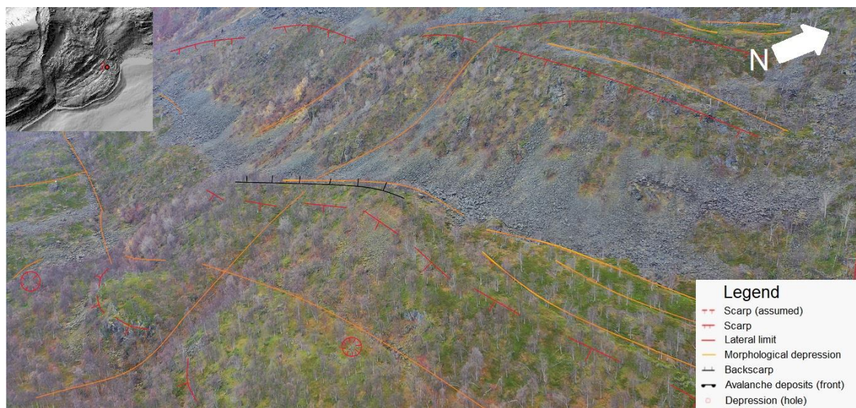
Figure 39: A map of the transition zone, on a 1:6500 scale, with morpho-structural elements found in the domain. Location is shown on map in the top left corner. Hillshade from 1 m DEM (Kartverket, 2021).
