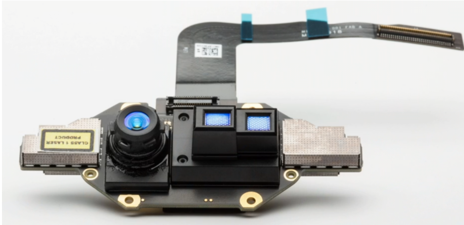
Figure 2.3: The Azure Kinect module separated from its housing [18].
