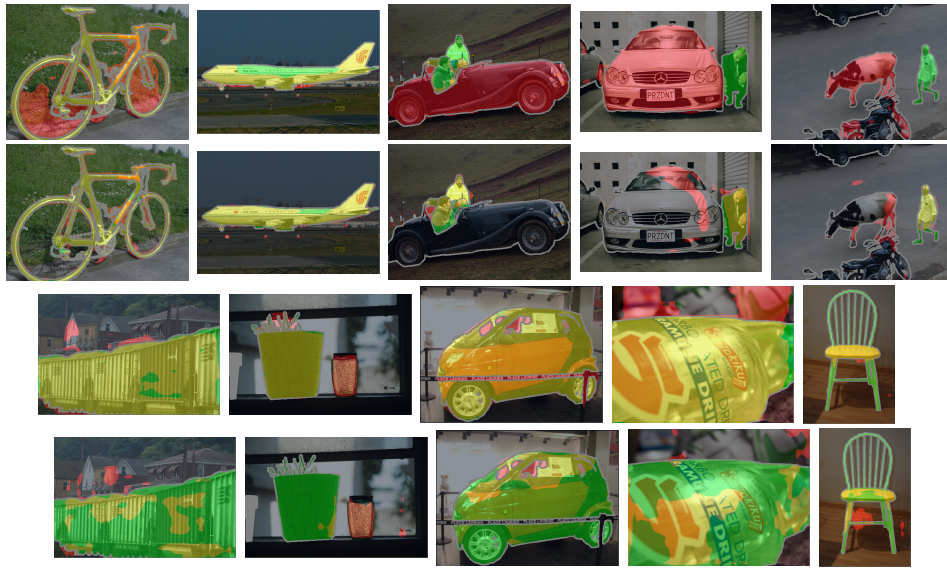
Figure 10.4: Example images before and after Inference Guided method. Here green is the true label that has not been predicted, yellow is true prediction, red is wrongly predicted areas and gray is ignored pixels. The first row is bad examples from the SGCG network that got improved with our IGFSS method in the second row. The third row is good examples from the SGCG network that got worse with our IGFSS method in the fourth row.
