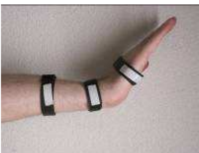
Figure 2.5. Reflective tape in the user's arm (Decker et al 2009)
