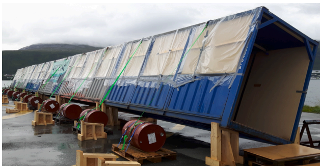
Fig. 1. The Tromsø test facility heeled at 20°.
