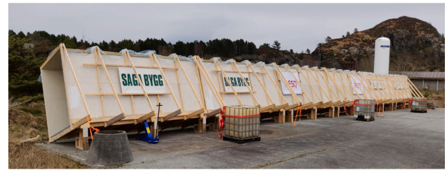
Fig. 2. The Haugesund test facility heeled at 20°.
