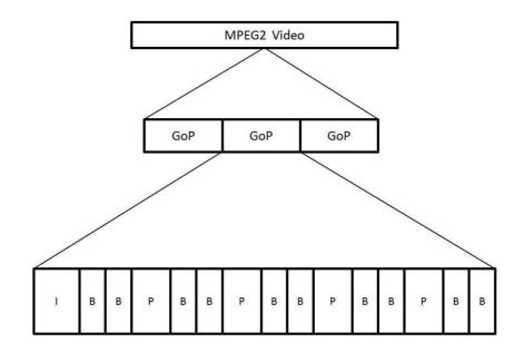
Figure 2.1: MPEG2 format Structure.
