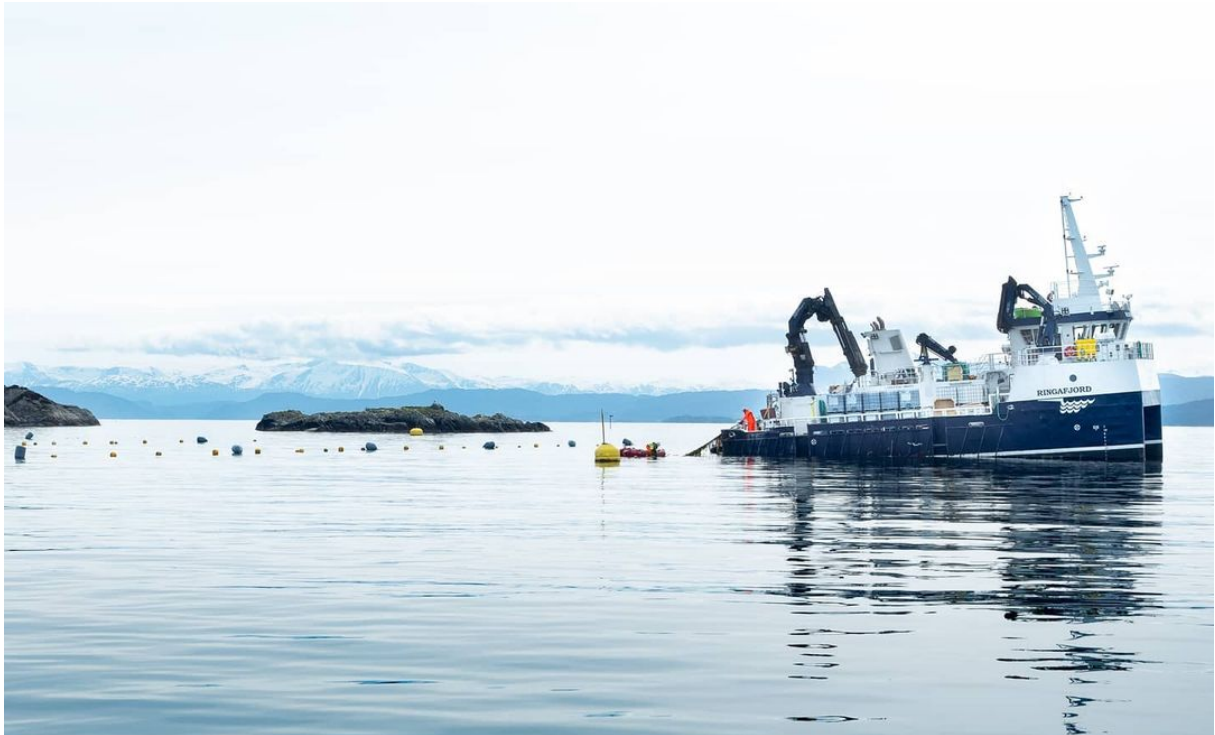
Figure 25 Heavy operation boat used in the Lerøy Ocean Forest farm (Norway). The boat is used both for harvesting and post-processing (fermentation). Source: Ocean Forest Instagram
