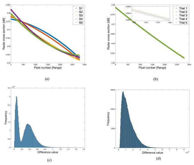
Fig. 2: (a),(b) Polynomial fits for the averaged profiles which were generated by taking strips of open water pixels and by randomly sampling the open water pixels respectively. The polynomial fits act as estimators for  $\sigma_{TR}^{0,sea}$  (the numerator in (1)). (c),(d) Histograms for the difference images. As can be seen, a greater degree of error is incurred by estimating  $\sigma_{TR}^{0,sea}$  using strips of open water pixels.
