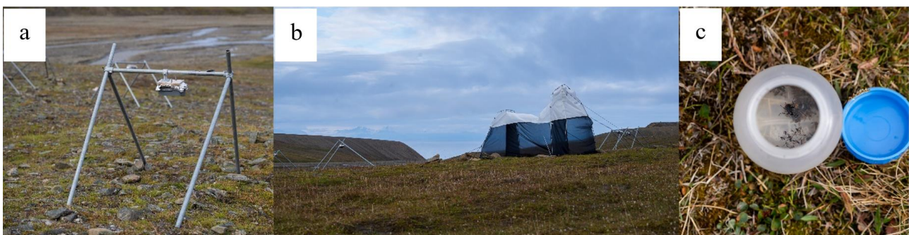
Figure 3. The field site in Bjørndalen. (a) Three steel mounted time-lapse cameras on top of Silene acaulis cushions, (b) the malaise tent next to the camera cluster, and (c) a combined sample from five pitfall traps. Photos: Line Klausen, 2021.
