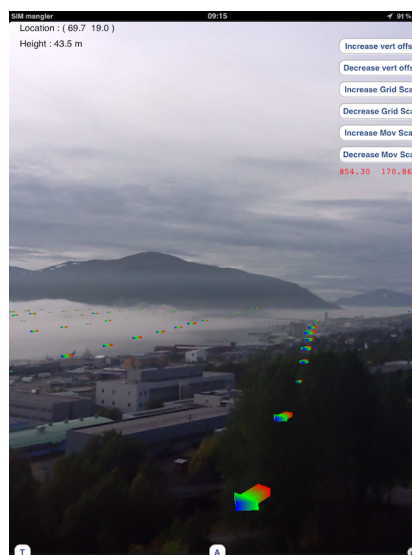
Figure 4: Screenshot of tablet with camera and an example of overlaid meteorological information
