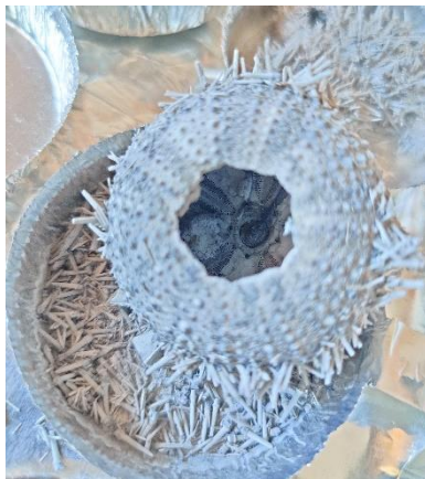
Fig. 6 All organic matter was burned in the muffle furnace. Only the empty shells remained.
