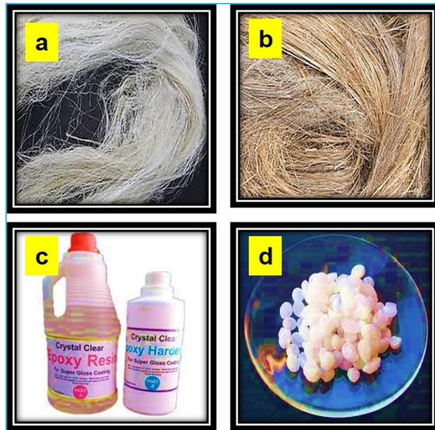
Figure 1. Photographic Images of (a) sisal fibre; (b) flax fibre; (c) Epoxy matrix; and (d) NaOH pallets.
