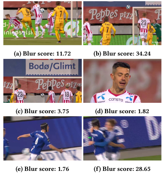
Figure 7: Results using the OpenCV Laplacian operator [3] on selected frames (higher score indicates less blur).
