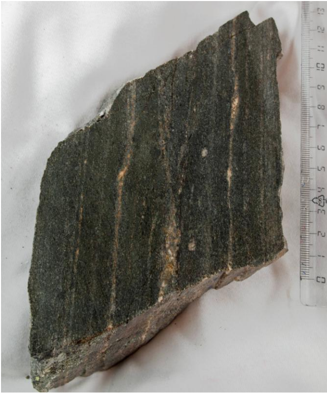
Fig. 2.8. Sample 8.1 representing Suborg-gabbro with a solid state overprint. A distinct layering is seen in this rock where alternating mafic- and felsic layers define a foliation.
