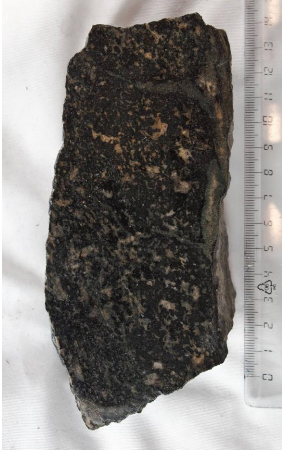
Fig. 2.12. Hand sample SuE-4 from magmatic lens. Notice large grain aggregates of felsic and mafic material with a somewhat preferred orientation.
