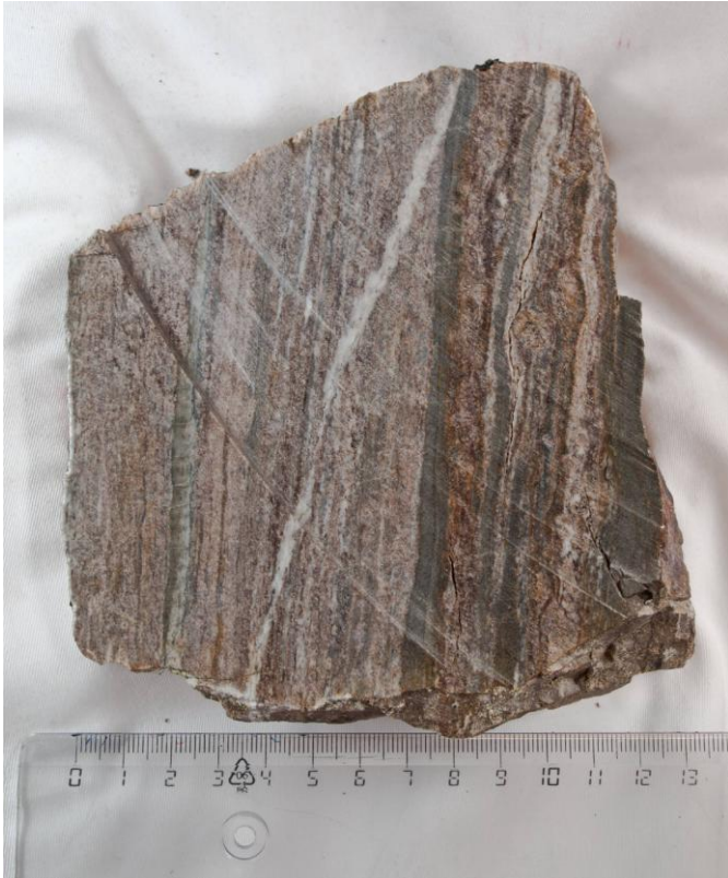
Fig. 2.16. Hand sample SuE-12 from a sheared quartz-feldspathic zone. The rock has layers rich in feldspars, biotite and garnet. Notice the steep fabric in the rock (the hand sample is oriented back to the field).
