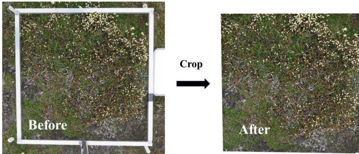
Figure 5. Example of a plot photograph taken with an RGB camera mounted 1.5 m above ground with a 75 x 75 cm aluminium frame. The frame and surrounding vegetation were cropped out before vegetation indices were extracted from the image. White flowers in the plot belong to the shrub Cassiope tetragona .
