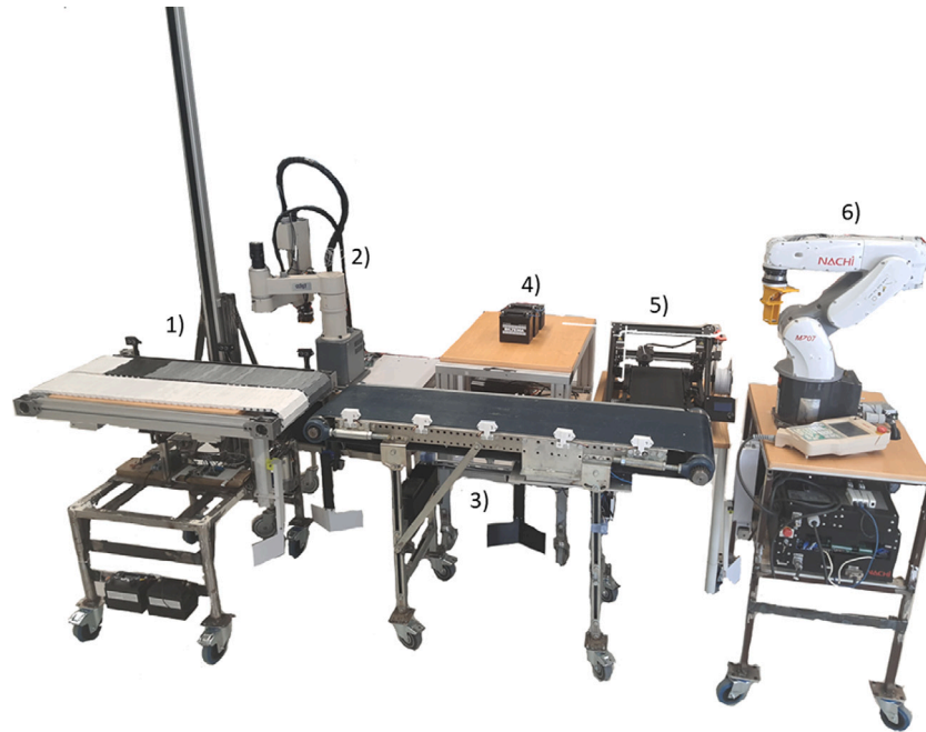
Fig. 4. The expansion of RMS with battery platform. (1) conveyor with lifting (2) Scara platform, (3) conveyor, (4) battery platform, (5) 3D printer, and (6) Nachi platform.
