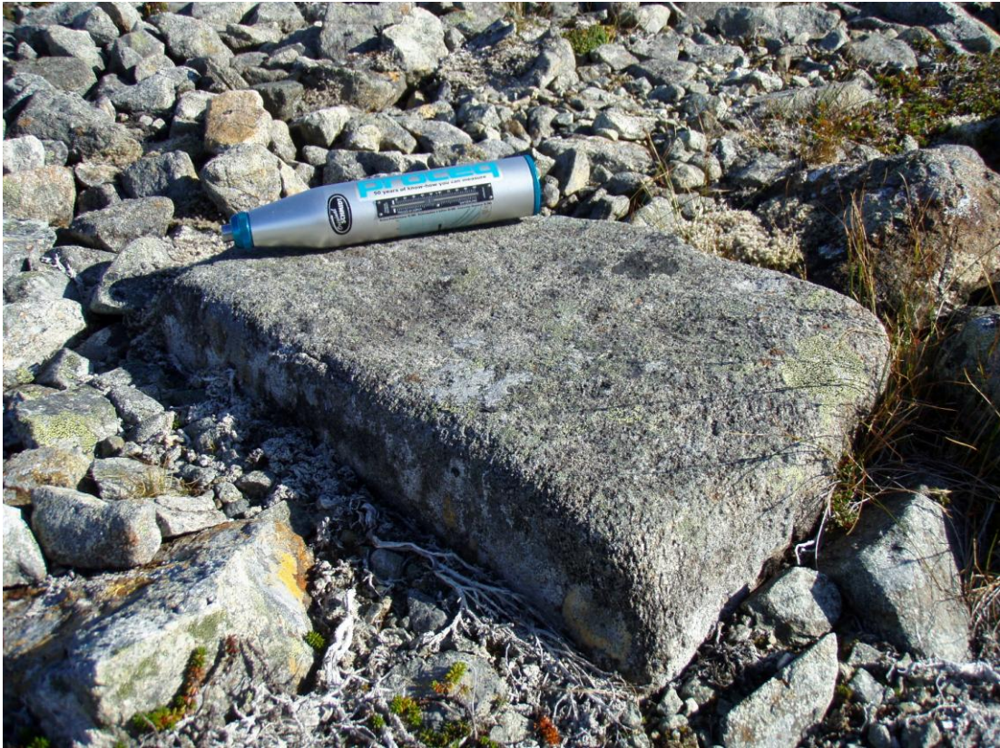
Figure 2.2.2.1. Proceq Schmidt hammer and ideal gabbro boulder.
