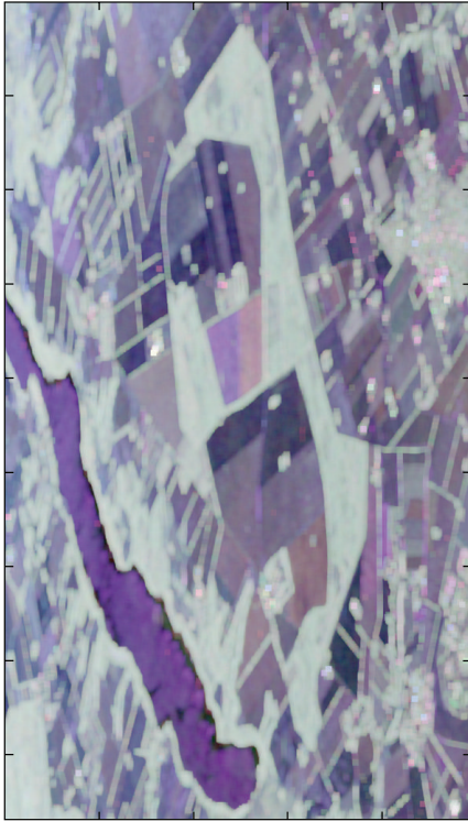
FIGURE 12: Polarimetry ( \Gamma matrix) image shown as Pauli RGB colours ( R = |HH - VV| , G = |HV| , B = |HH + VV| ).
