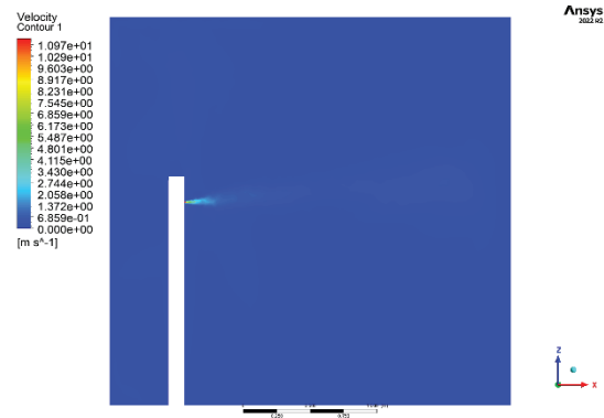
Fig. 13. Velocity contour for turbulence model RNG k-\epsilon
