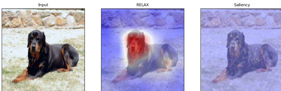
Fig. 4 Comparison of RELAX and saliency explanation for an image from PASCAL VOC. The example shows how both explanations focus on the dog, but the saliency explanation is much more erratic and unfocused than the RELAX explanations
