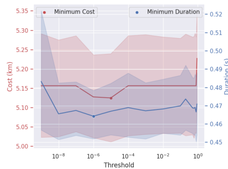
Figure 6.4: Threshold experiment performed to find the optimal tradeoff between computational time and cost.
