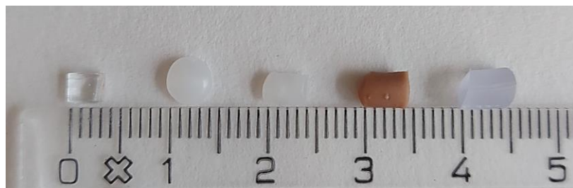
Figure 6: Microplastic polymers used in the thesis. From left; HDPS, HDPE, PP, PVC B, and PVC A.
