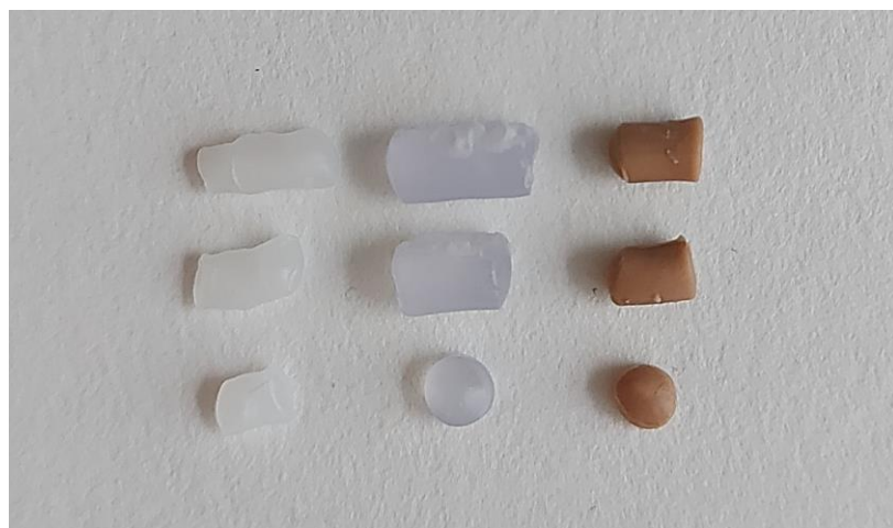
Figure 7: Different characteristics within the same microplastic polymer. From left; PP, PVC A and PVC B.
